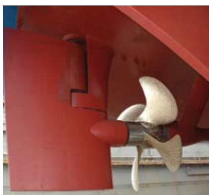
Installation complete – Prefabricated bulbs welded to the existing rudders.
